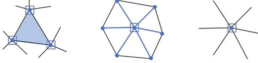
Fig. 6. Vanka Subdomains. The pressure DoFs are illustrated using squares and the position DoFs are illustrated using dots. The cell-oriented Vanka (left) uses both position and pressure DoFs in a cell as a subdomain; The patch-based Vanka (middle) uses a single pressure DoF and all connected position DoFs as a subdomain. Our vertex-based Vanka (right) uses only the position and pressure DoFs associated with a single vertex as a subdomain.
